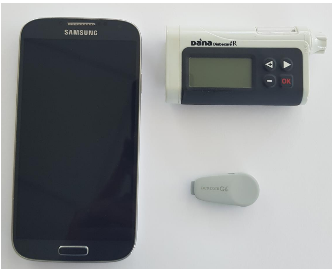
Figure 1A CamAPS FX comprises Samsung Galaxy phone (or similar) running Cambridge control algorithm, Dana insulin pump (Sooil), G6 real-time CGM sensor (Dexcom).
