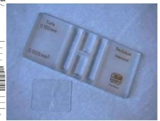
6. Place the chamber beneath a x25 objective and bring the sperm into focus on the first (1) of the corner squares (1, 2, 3 or 4). Switch to x40 and using a manual counter, count the cells in the square, moving from left to right, row by row and omitting cells contacting the right and lower edges (red crosses). The example below
