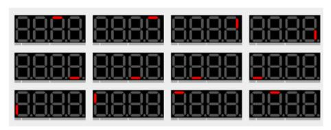
Step off the scales and wait for dashes to appear on the display, this means the measurement is being transmitted. Once the measurement has been successfully transmitted, the lines will show a box like the image below.
