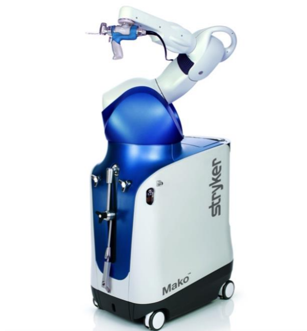
Figure 1: The MAKO robot. The surgeon moves it into the surgical field, the robot controls the cuts
