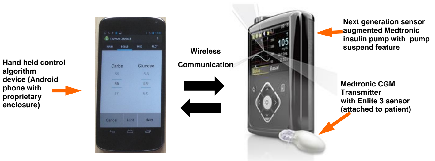
Figure 1: Representative design of the proposed FlorenceM automated closed loop system
